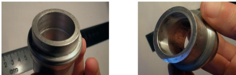
Figure 17. To the elimination of dimples in the zone of extrusion of the outer flange with the help of technological shoulder
